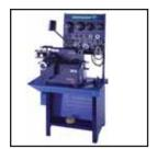
Combination brake lathes for rotors, drums, and flywheels.
